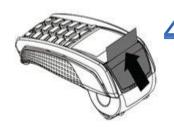
While your terminal is displaying the idle screen, press and hold the YELLOW button to ensure that the paper feeds correctly. Attempting to fit rolls of a different size may damage your terminal.
