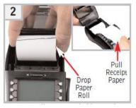
Unstick the end of the new roll. Leaving the end free, hold the paper roll and carefully place into the printer compartment.
